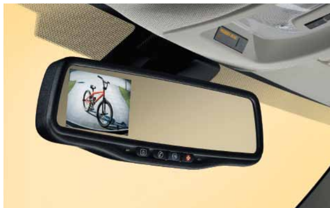
A REAR-VIEW CAMERA IN THE 2011 CHEVY EQUINOX DISPLAYS IMAGES ON A MONITOR CONCEALED IN THE REAR-VIEW MIRROR.
