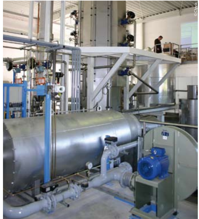
The smaller of the Clyvia production plants can produce 500 liters of diesel per hour.
